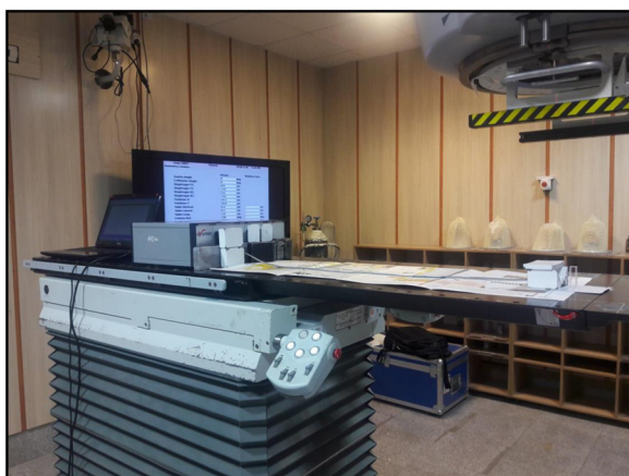
Fig. 1. The set-up of photo-emission recording during X-ray irradiation by a Linac.
